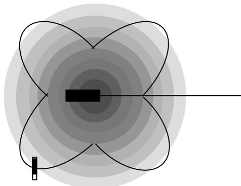
(B) When antenna and tag are perpendicular with each other
